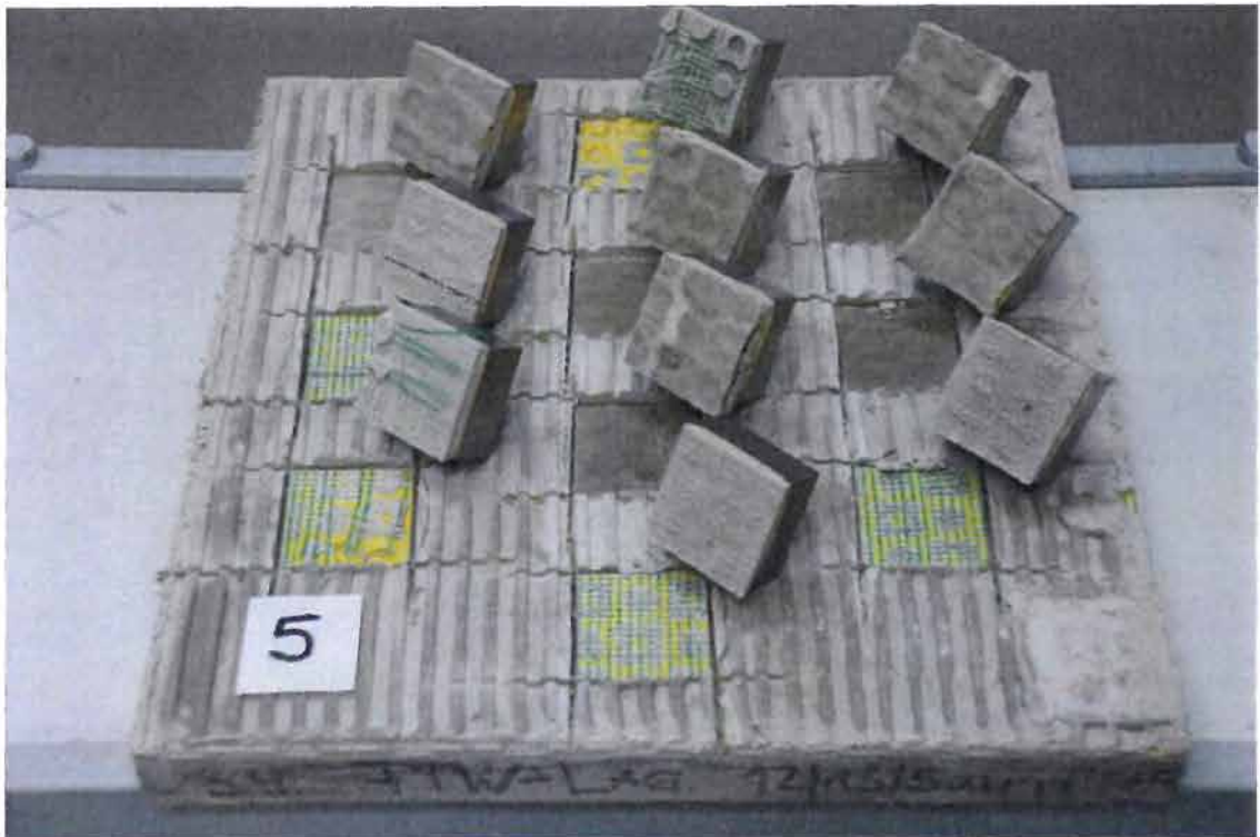
Figure 10.: Slab with DURABASE CI++ rolled-up mat and Sopro megaFlex S2 after exposure to freezing and- thawing and after the adhesion test
