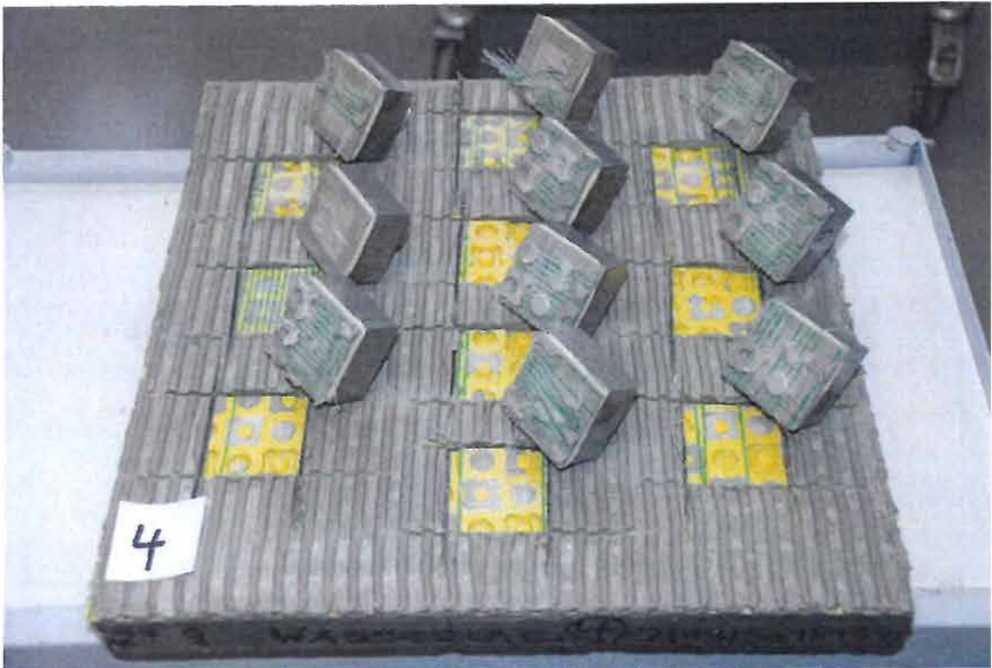
Figure 8.: Slab with DURABASE CI++ rolled-up mat and Sopro megaFlex S2 after water immersion and after the adhesion test
