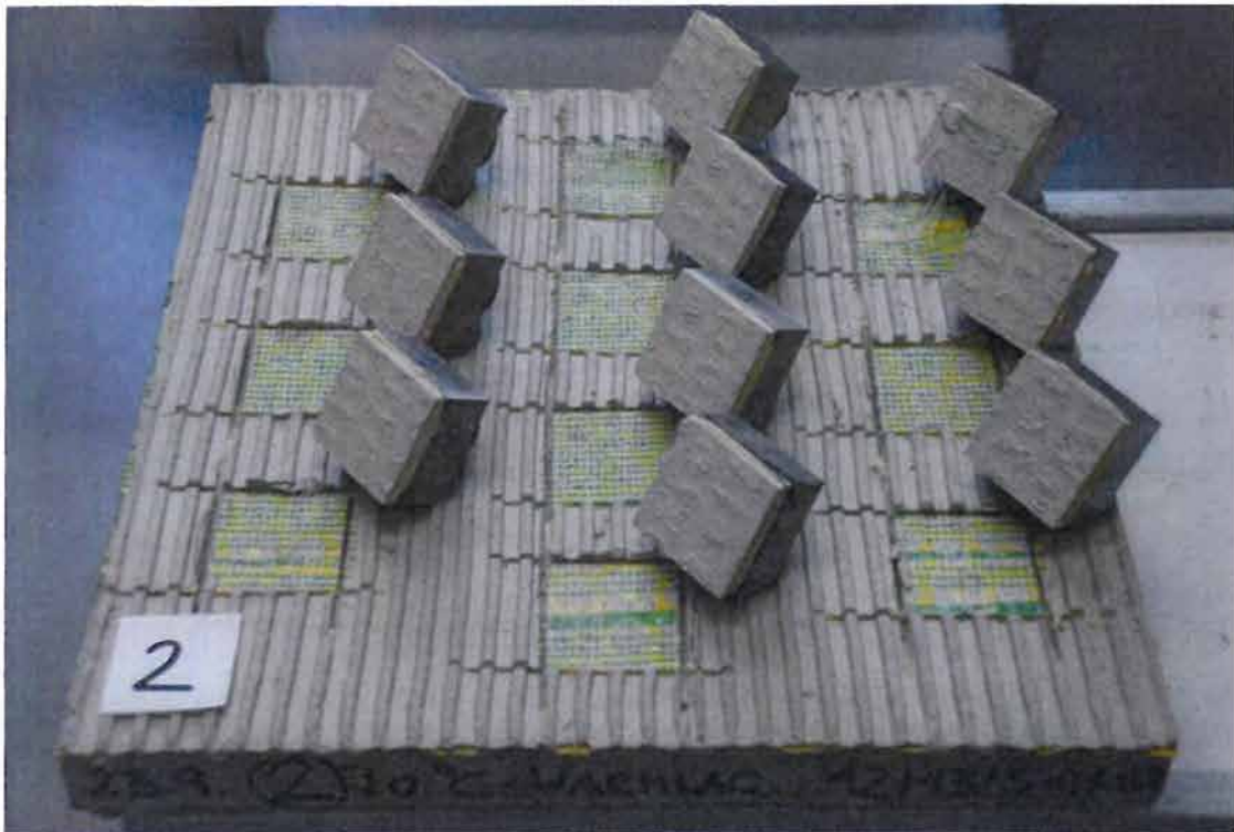
Figure 6.: Slab with DURABASE CI++ rolled-up mat and Sopros No.1 flexible adhesive after heat exposure and after the adhesion test
